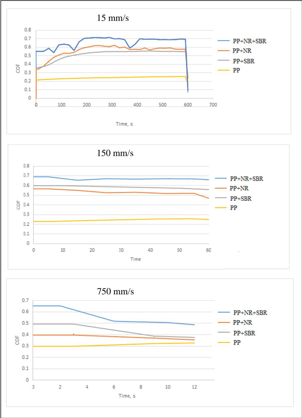
Fig. 3. Coefficient of friction measurements for different samples and sliding speeds.
