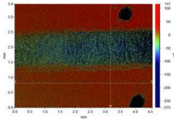
Fig. 2. Optical interferometry image of the track in PP-NR at the 150 mm/s sliding speed.
