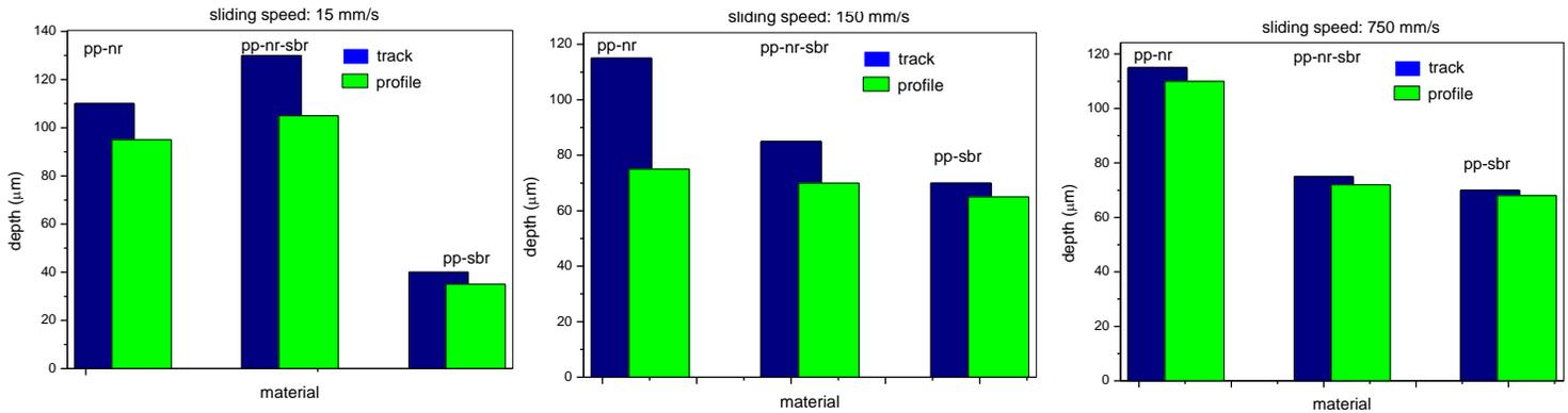
Fig. 1. Maximal track depth and track profiles for different samples and sliding speeds.
