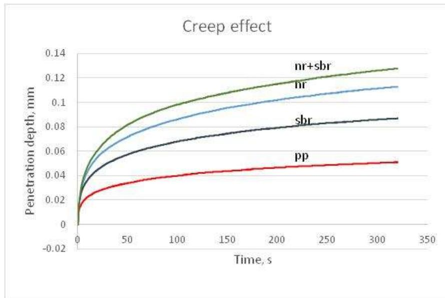
Fig. 4. Creep effect measurements for different samples and the sliding speeds.
