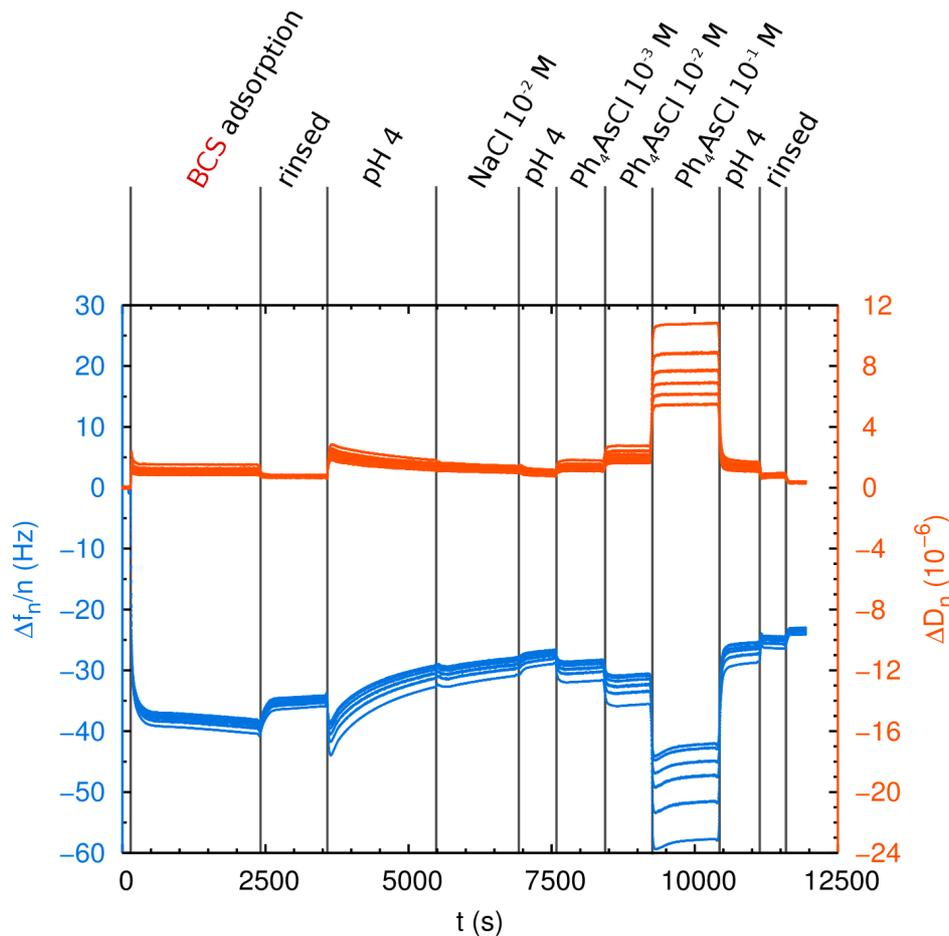
Figure 5: QCM-D: changes in resonance frequency (blue) and dissipation signal (orange) for different harmonics for different stages of adsorption and rinsing, as indicated. The hydrophobic ion  $\text{Ph}_4\text{As}^+$  acts as co-ion.
