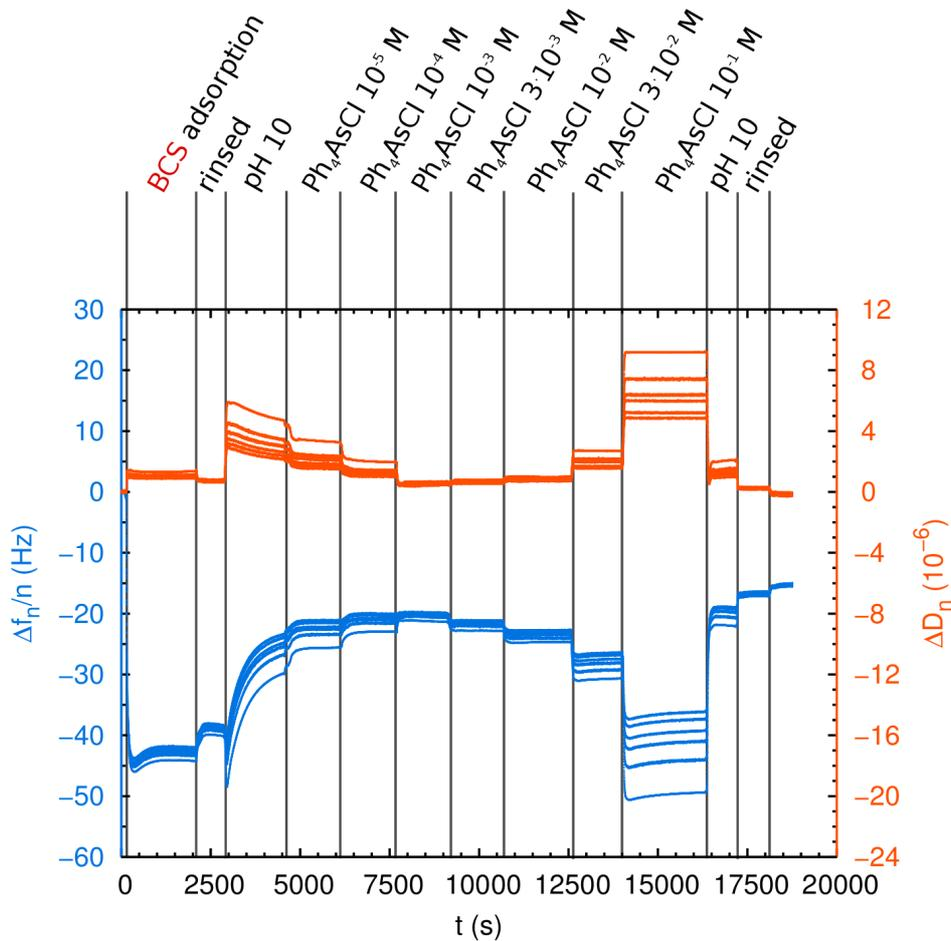
Figure 4: QCM-D: changes in resonance frequency (blue) and dissipation signal (orange) for different harmonics for different stages of adsorption and rinsing, as indicated. The hydrophobic ion  $\text{Ph}_4\text{As}^+$  acts as counter-ion.
